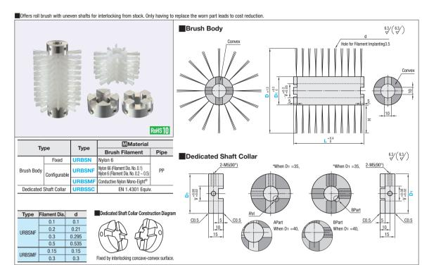
🕐 Use the brush at less than 1000rpm (the maximum rotation for URBSMF is 400). Note that maximum rotational speed varies depending on the mounting method, the brush length, the brush 0.D. or the number of connected brush.
