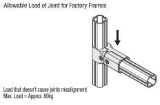
Please note the maximum load is the value of the static load, and impact load may be lower than this value.
